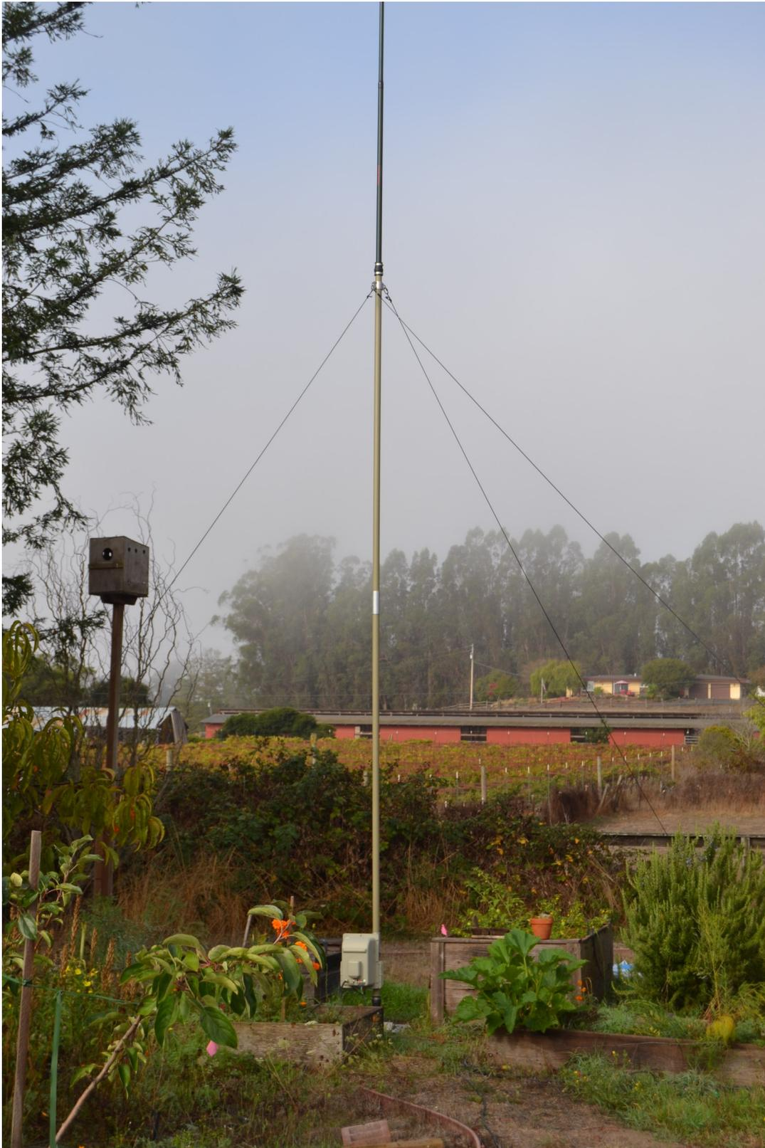
Big IR Mark III at K6SRZ. This allowed us to have a resonant antenna on both 75 and 80 Meters. A brand new antenna and only used for about an hour during CQP. BTW, it's for sale!
