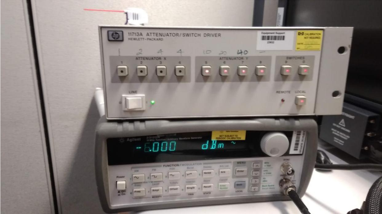
Power out is now -20.119 dBm with in at -6 dBm. Only about 2 dB of change over 106 dB of change on the input. The magic func(on of an AGC.
