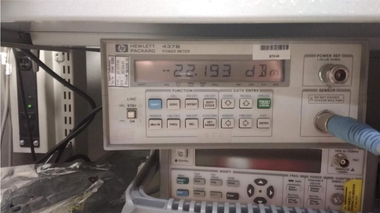
All steps are disengaged here, and signal generator is set to -6 dBm a change of 106 dB from previous picture.
